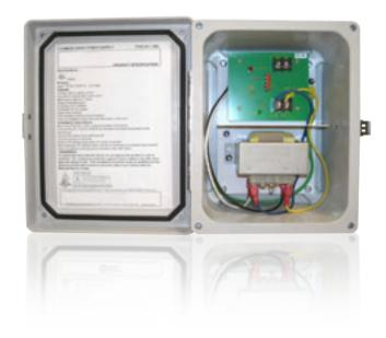
The PWR-24AC-1-3-ULW is a CCTV power center engineered to manage remote camera and accessory power requirements in a NEMA 4X weatherproof enclosure. The PWR-24AC-1-3-ULW distribution module is designed with 1 individually fused output for powering up to 1 CCTV camera or accessory. It will provide 24Volts AC via distribution to one fused output with a total of 3.0 Amps continuous supply current.
