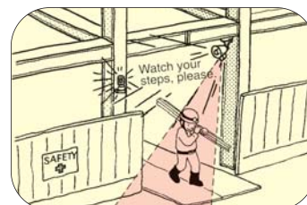
●Alarm/warning speaker at constructions site
