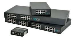
Pace PRM Series Receivers Up to Sixteen (16) Port IP and PoE+ Receivers Transmit IP video/data over CAT5e up to 500m @ 100Mbps. Support PoE (IEEE 802.3af) or PoE+ (IEEE 802.3at). UL/cUL Listed (UL60950-1). CE and C-Tick Approved.
