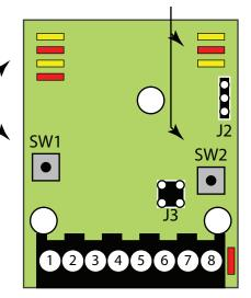
5VDC - 12 VDC Reader Power Jumper
