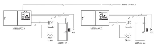
**MiniMax 3** – The MiniMax 3 configuration is ideal for applications where the doors are far apart and/or the control is located at the door.
