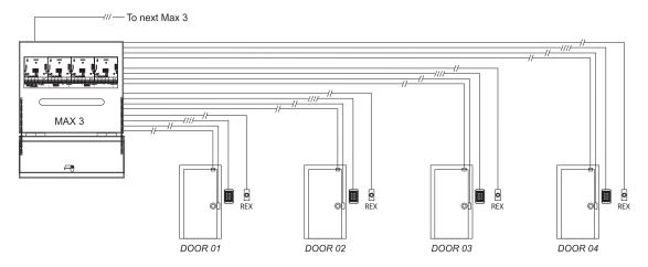
**Max 3** – The Max 3 cabinet configuration provides the simplest expansion of one to four doors per cabinet when the system needs to be installed in a central location.
