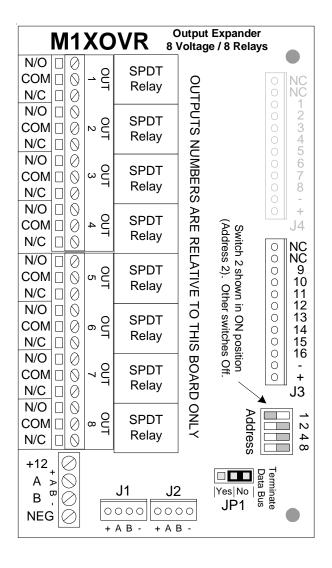
ADDRESS SETTING: Locate the four "Address" switches. Each has a position of OFF or ON (binary 0 or 1) with a decimal equivalent of (1, 2, 4, or 8). The total decimal value for the "ON" switches sets the bus address. This determines which outputs (banks of 16) are assigned to the expander. E.G. Address 5 would be set with switches 1 and 4 ON (1+4=5) and switches 2 and 3 OFF. Outputs Expanders are factory pre-set to address 2 (Outputs 17 to 32).
