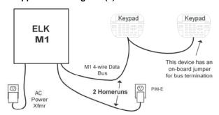
Ideally the M1 should have no more than 2 Data Bus home runs. The end of each homerun should terminate with a 120 Ohm resistor. Many M1 devices have a jumper for this purpose. See other wiring diagrams.
