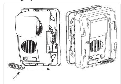
Gentex Super-Slide<sup>®</sup> Mounting Bracket: Allows the installer to pre-wire the system, test for system supervision, remove the signal head until occupancy, switch out Gentex signals without changing mounting brackets and has locking edge connector for snap-in-place installation.
