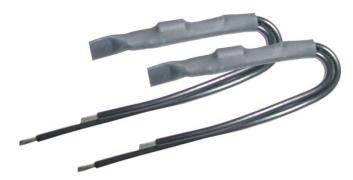
**DITEK's DTK-ESS** protects electric door strikes. Electric door strikes (magnetic locks) are typically installed in metal frames, with low voltage wiring back to an access control panel, creating a vulnerable surge path. The compact ESS installs in the door frame to prevent voltage surges from getting into the control panel.
