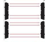
Require extra protection at the perimeter? Choose a photobeam detector that has four channel selectable frequency and stack two of them on a pole or better yet, in an AX-TW200 Beam Enclosure.
