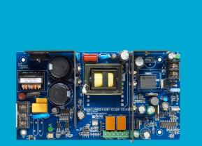
The Securitron AQS1210 Series of switching power supplies are single voltage, UL listed, supervised units with a dedicated battery charging circuit. They provide 10 Amps at 12VDC, with up to 16 independently controlled power limited outputs.
