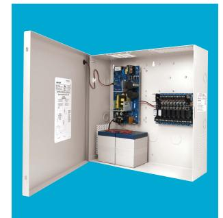
The Securitron AQD2 Series of switching power supplies are dual voltage, UL listed, supervised units. These units are field selectable with a dedicated battery charging circuit. They provide 2 Amps at 12VDC or 24VDC continuous, with up to 16 independently controlled power limited outputs.
