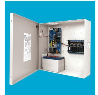
The Securitron AQD1 Series of switching power supplies are dual voltage, UL listed, supervised units. These units are field selectable with an integrated battery charging circuit. They provide 1 Amp at 12VDC or 24VDC continuous, with up to 16 independently controlled power limited outputs.
