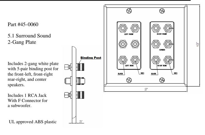
Installs in a NEMA 2-gang box or low-voltage mounting bracket.
